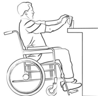
Figure 2: Vertical positioning of counter mounted PED for disabled user
